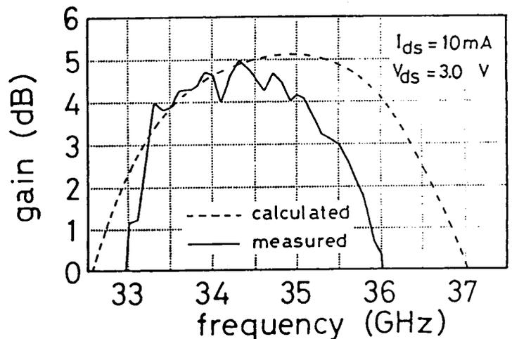
FIG. 4 Calculated and measured gain characteristics of the fabricated amplifier
