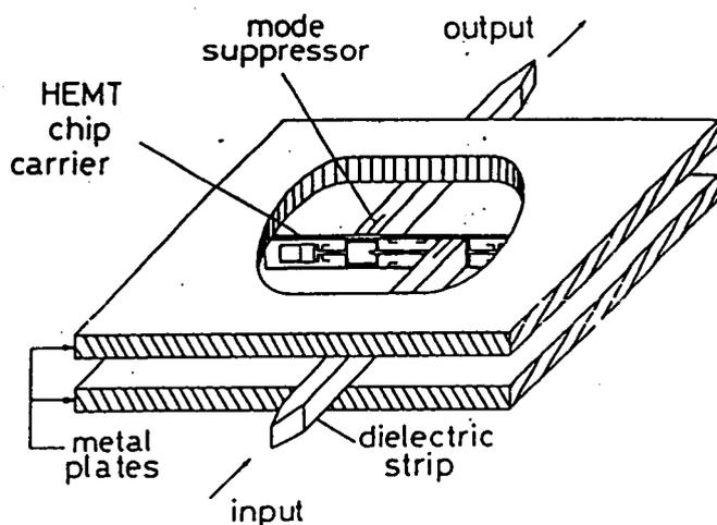
FIG. 1 View of the NRD guide HEMT amplifier
